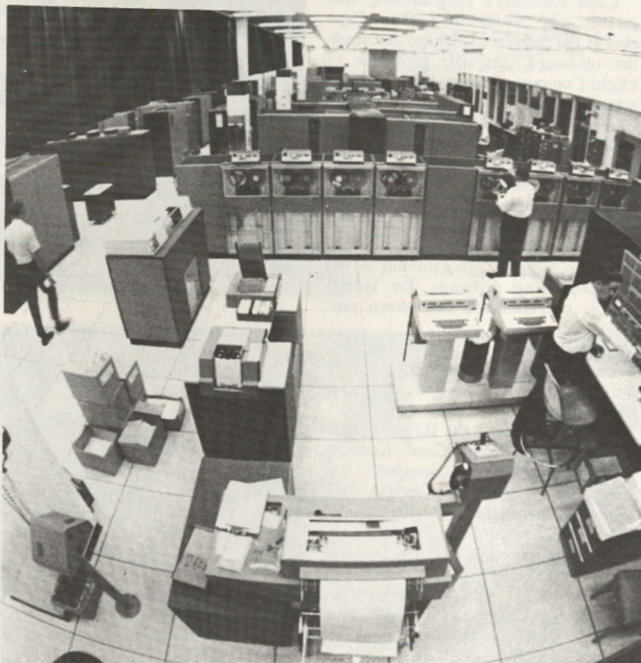
Five IBM System/360 Model 75s in Houston's Real Time Computer Complex keep track of mission detail for flight controllers and astronauts.
