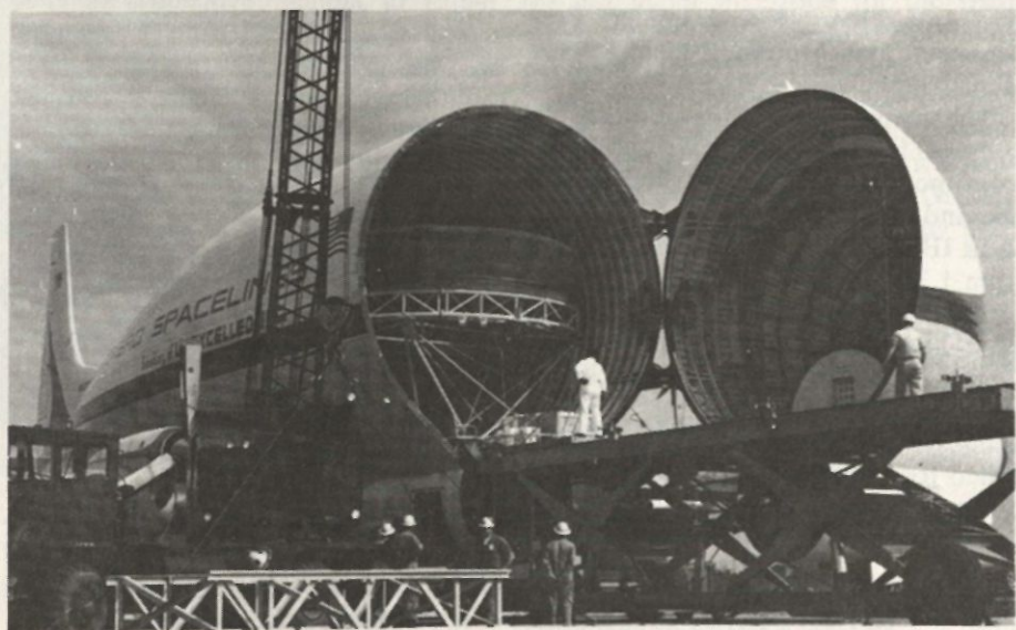
Draped and mounted on a traveling cradle, the IU nests in the Super Guppy at the start of a journey from Huntsville to the Cape.
