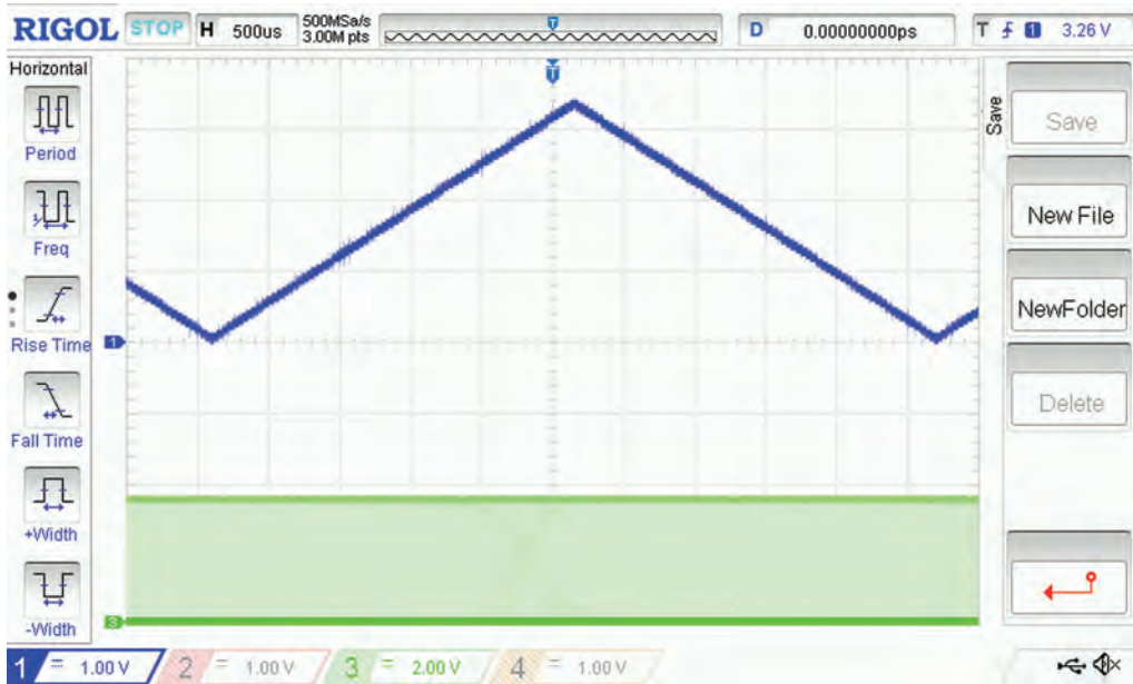
Figure 7.15 Output of ISR-based triangle waveform generator program. Upper trace is DAC output, lower trace is ISR activity (Port D bit 1).
