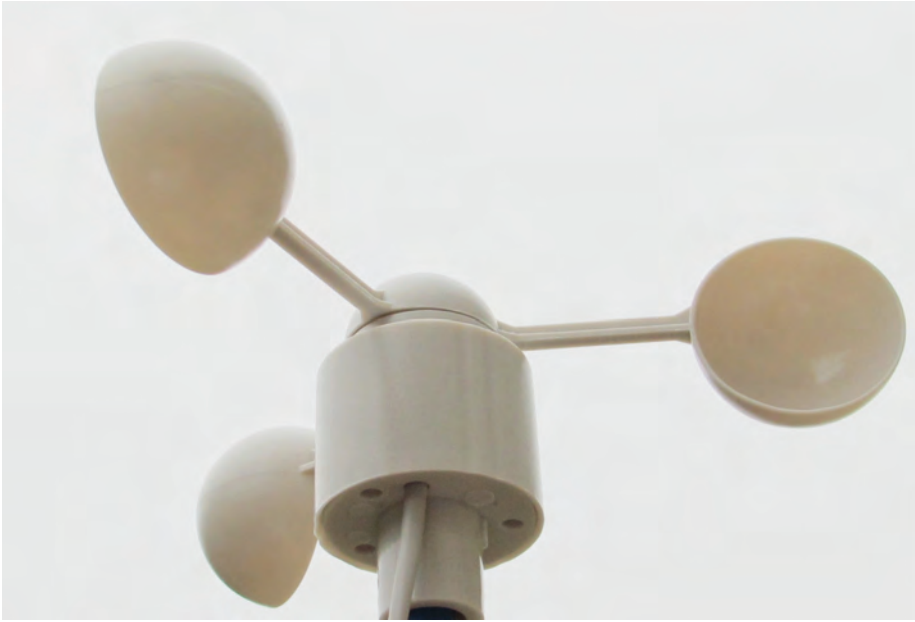
Figure 7.2 Cup anemometer used to measure wind speed. Photo by author.
