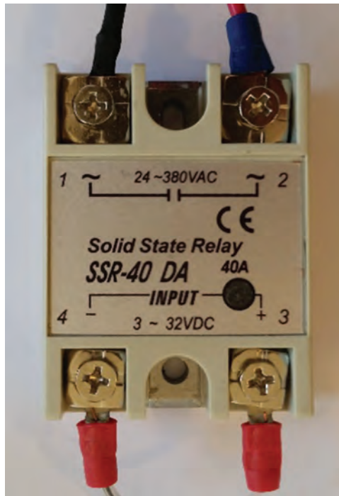
Figure 2.16 A solid-state relay allows the MCU to switch devices powered by up to 380 V AC.
