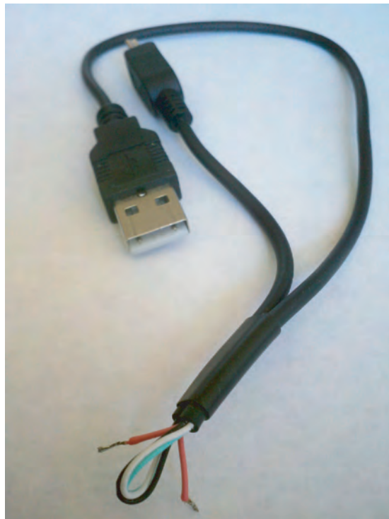
Figure A.3 Modified USB cable allows measurement of entire board’s current draw.
