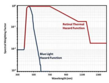
Figure 1: Retinal thermal and blue light hazard functions
